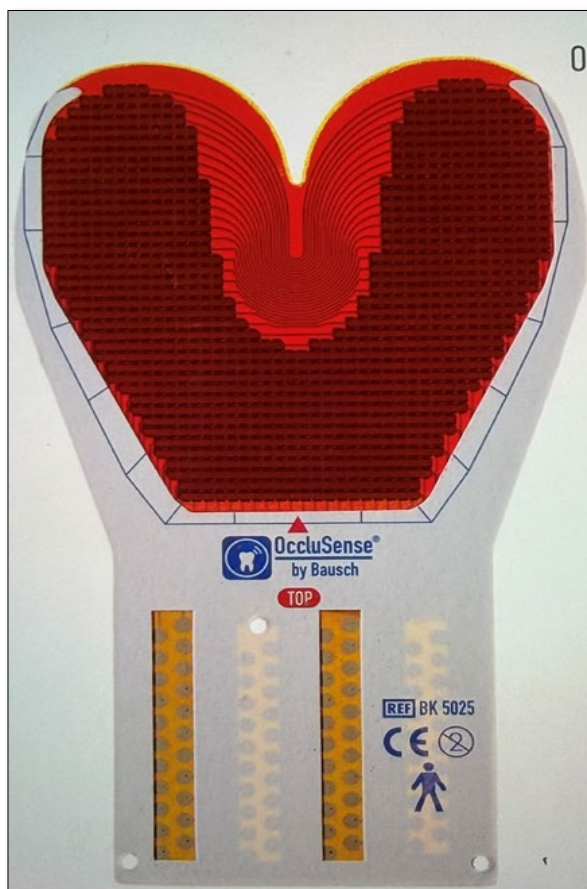
Figure 1. A plastic wafer is shown with sensors. It is semi flexible and 60 microns thick. The underside can be used as a contact indicator.
