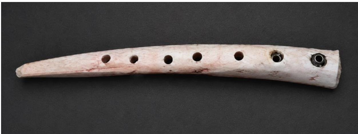
Figure 2. Cortical view of the bovine rib after implant placement and attempted retrieval. Five implant-bed sites are visible following successful implant removal. The implants positioned at sites 1 and 2 remained embedded after failure of the implant–driver hexagonal engagement during counter-torque retrieval. These sites were excluded from elemental analysis because removal would have required trephination or sectioning of the surrounding bone, potentially disrupting the specimens and introducing additional metallic debris.
