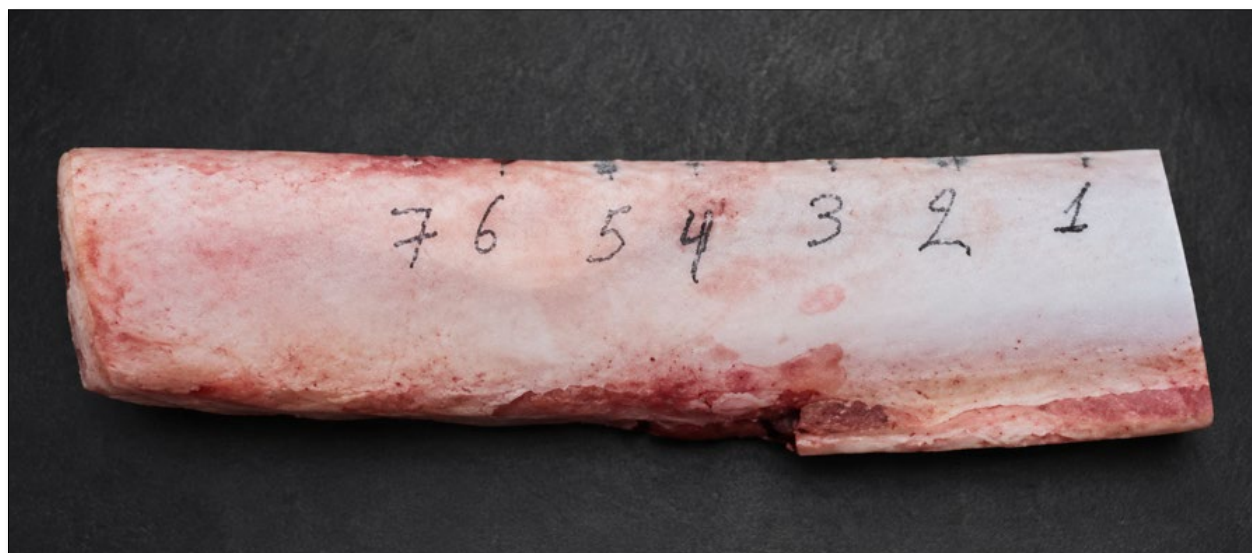
Figure 1. Identification of the experimental implant sites in the bovine rib segment. The seven placement sites were sequentially labelled from 1 to 7 to maintain correspondence between each implant system, its retrieval outcome, and the coded bone specimen submitted for elemental analysis.
